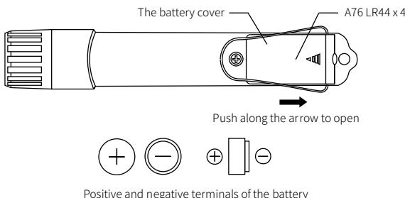
Install the batteries according to the positive and negative (  $\oplus\ominus$  ) in the battery slot.
